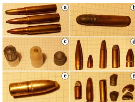
Fig. 1: Ammunition for small arms: a – bullets, calibre 30 06, with different projectiles: a FMJ at the bottom and two JSP above; b – a jacket-less projectile of old type; c – ball ammunition for smooth-barrel guns; d – projectiles for hunting guns; e – a JSP with the element made of polymers in the top segment; f – ammunition for handguns, from the left: two bullets for pistols, the first one with a cross-section of a projectile, a shell of a revolver bullet, and three deformed projectiles. Scale: one square = 0.5 cm. Figure from authors collection.
